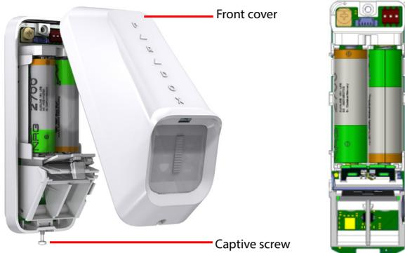
Figure 1 - Removing the Front Cover
